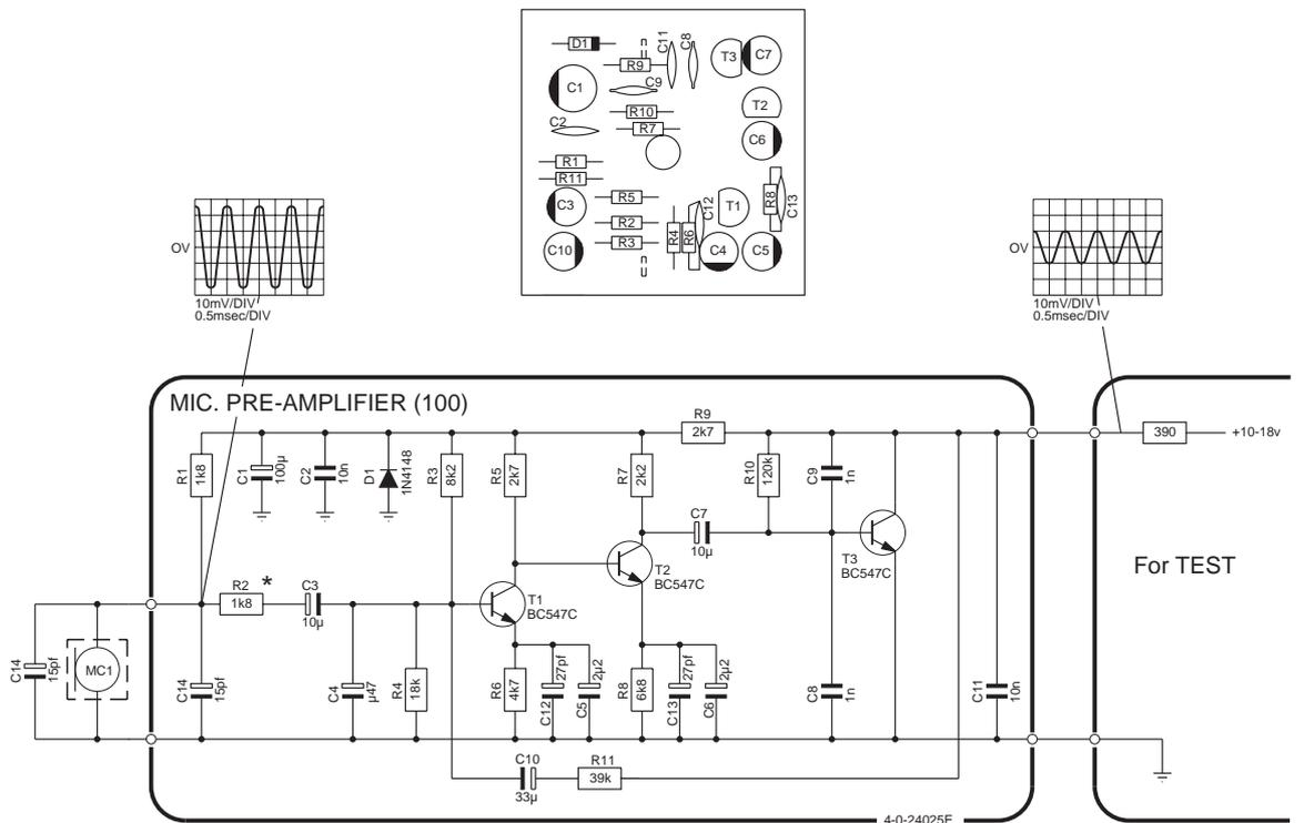
\* In orange marked microtelephone cartridge, R2 is changed from 1k8 to 5k6 ohm.
