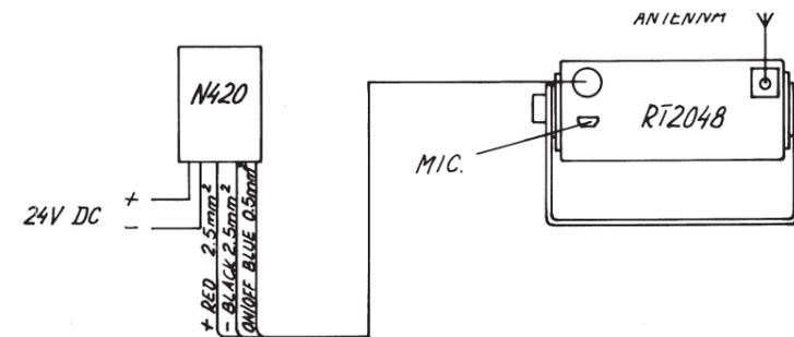
BLOCK DIAGRAM OF STRAPPING FOR 24V DC
