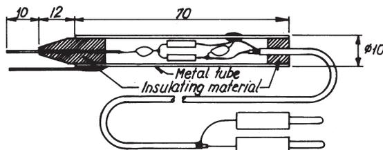
All measurements made by means of a test probe will be relative measurements. For quantitative measurements the diode probe should be calibrated by means of a signal generator at a certain impedance level (50 ohm) as a function of frequency.
