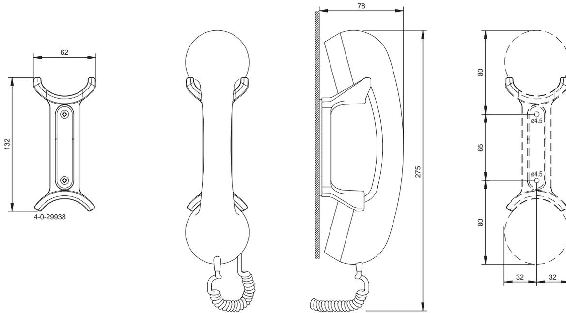
**MECHANICAL DIMENSIONS FOR HANDSET HOLDER WITH MICROSWITCH**
