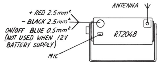
BLOCK DIAGRAM OF STRAPPING FOR 12V DC
