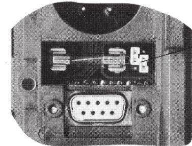
Strap for connection to external supply (12V)
