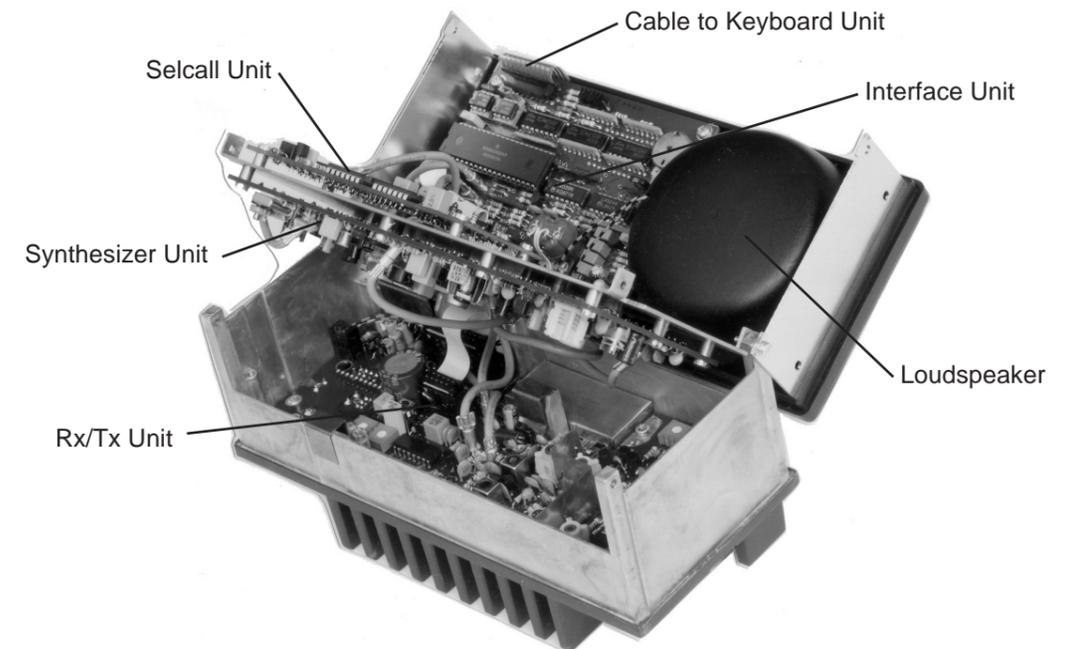
**4.1. MECHANICAL DISASSEMBLING RT2048**
