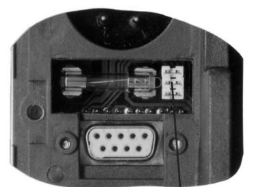
Strap for connection to external supply (12V)
